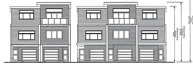
2 Units 1-5 SOUTH Elevation Scale: 1/8" = 1'-0"
